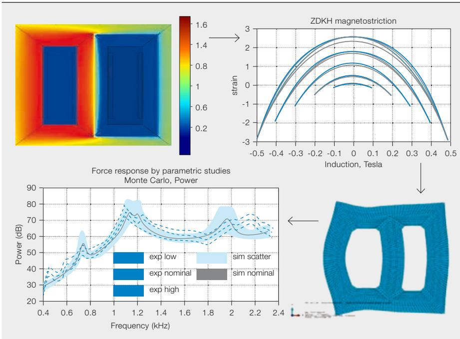
structure and finally sound power levels, which present a good agreement with measured levels, are shown in → 4.
