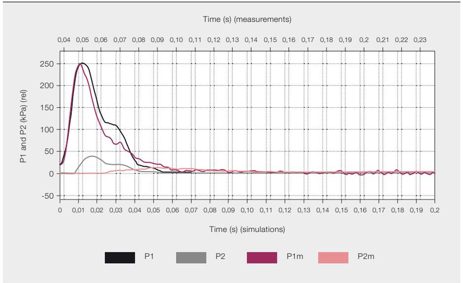
Type tests not only verify that the switchgear enclosure withstands the pressure, but also prove that hot gases are directed away from personnel.
