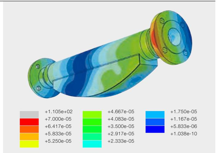
3b Under a strong external static load (axial torque)
