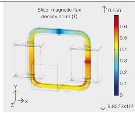
**8b** Respective instantaneous magnetic flux-density distribution (absolute value) in the center plane of the transformer core
