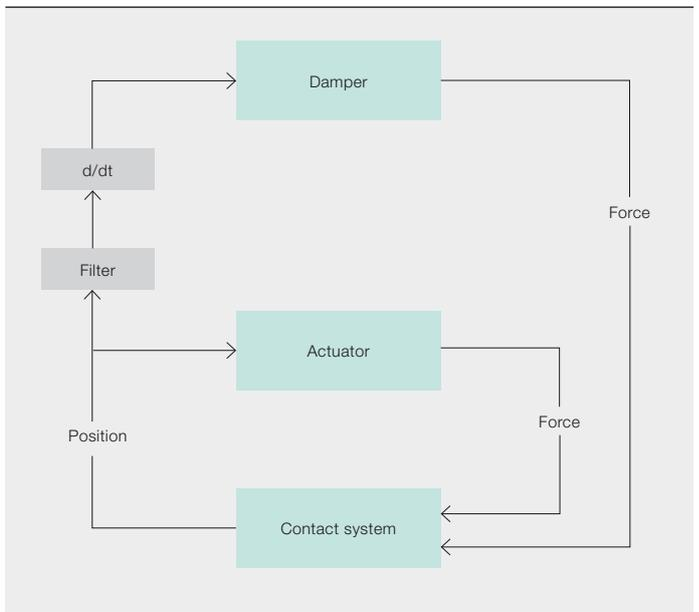
The Thomson effect uses the mutual inductance between two electrical conductors, creating a strong time-variant repelling (Lorentz) force between the conductors.
