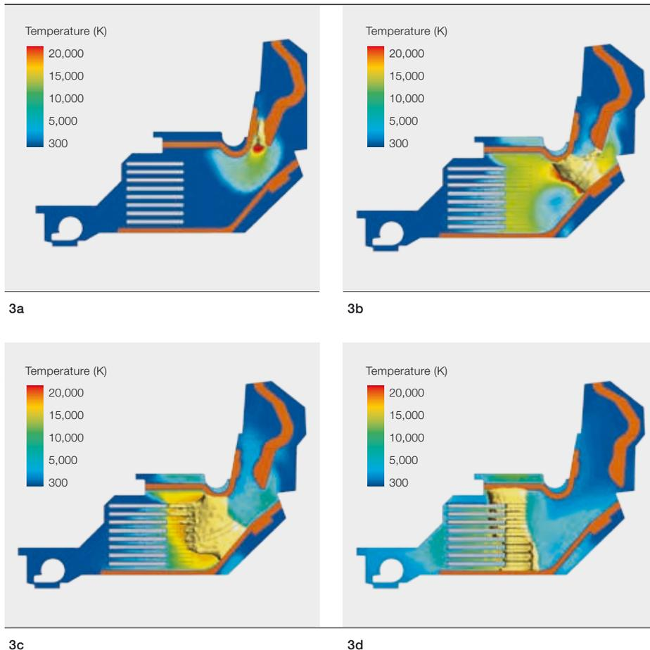
It is necessary to precisely simulate the flow conditions and the electro-magnetic forces that influence the shape of the arc.
