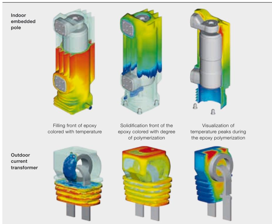
ABB uses advanced computer simulations in all of its polymers processing technologies, including reactive molding, injection molding, and silicone molding.
