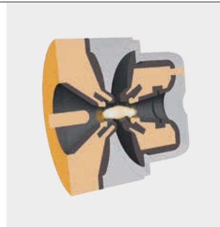
1b The plug has moved out, the breaker is in the fully open position and the arc burns between the contacts.
