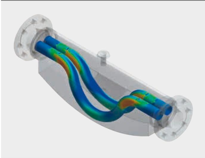
2a Operational eigenmode: deformations and stress distribution
