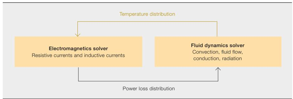
6 A coupled electromagnetic/thermal computation for a low-voltage busbar system
