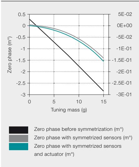
For the gray and green curves, the right y-axis, which is scaled up by a factor of 10, applies. The symmetrized design has a zero point that is much more stable under mass differences between the twin tubes.
