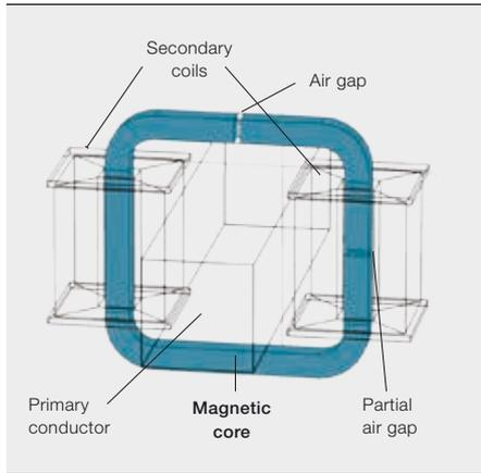
ric model can be modified, and it can be extended with a flux sensor in one of the gaps and with electric circuitry to form a closed-loop current sensor.
