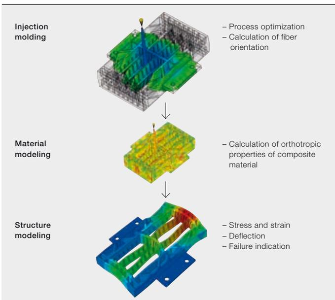
Advanced computer simulations are conducted in order to optimize each part and mold design before mold fabrication.
