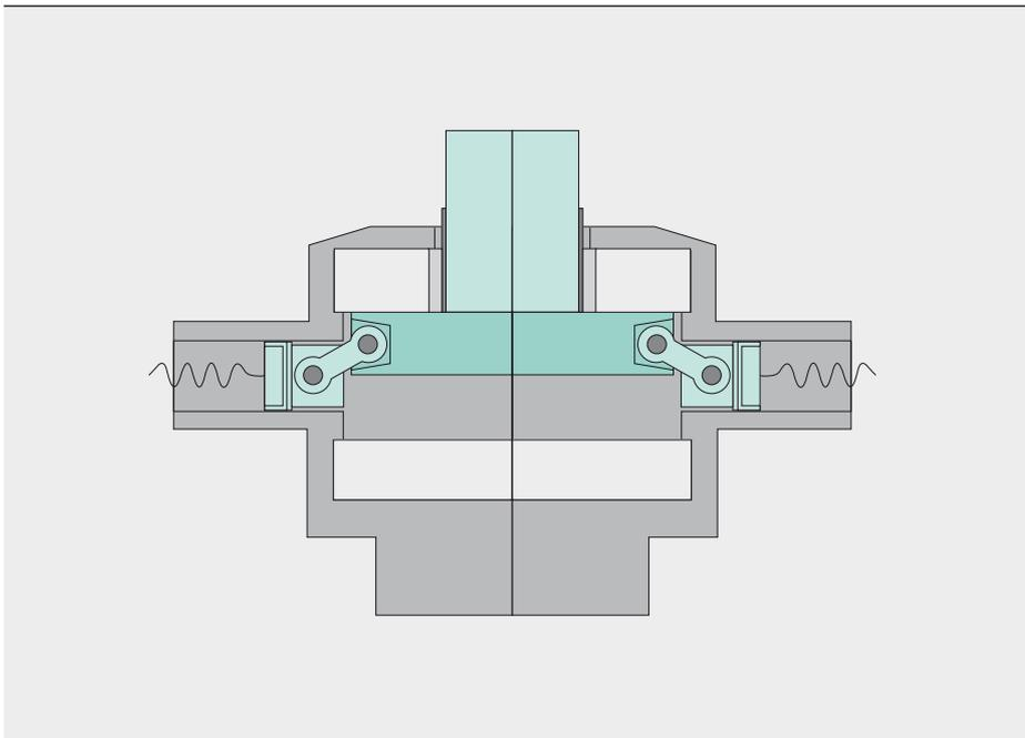
The UFD has to be able to transition from carrying full current load to providing high-voltage insulation within a few milliseconds.
