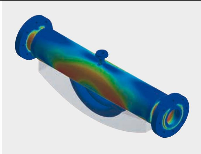
2b Stress distribution for the lowest eigenmode of the device's housing
