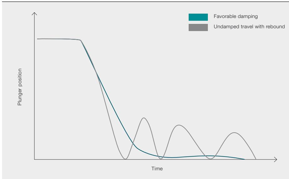
One big challenge for the design was to get good damping for both opening and closing operations without dissipating energy during acceleration.
