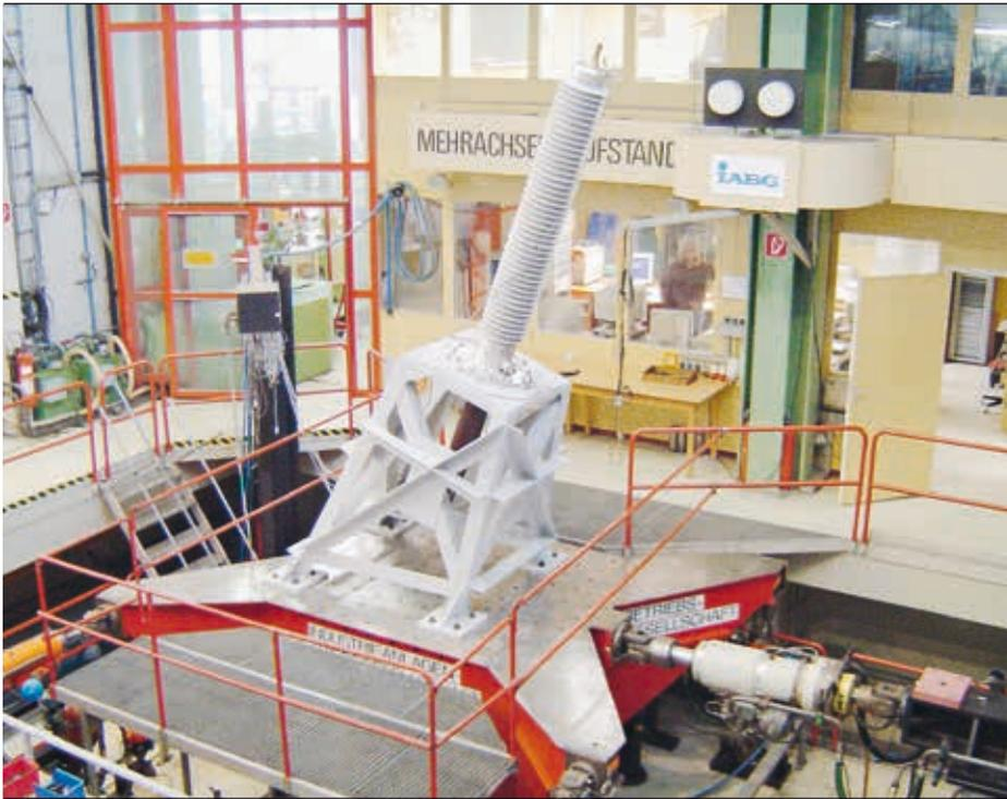
1a RIP 230 kV bushing under seismic test
