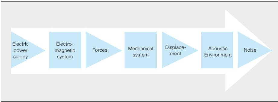
This simple model will predict the noise produced by capacitors on site with an accuracy of  $\pm 1.5$  dB, long before any component is built.
