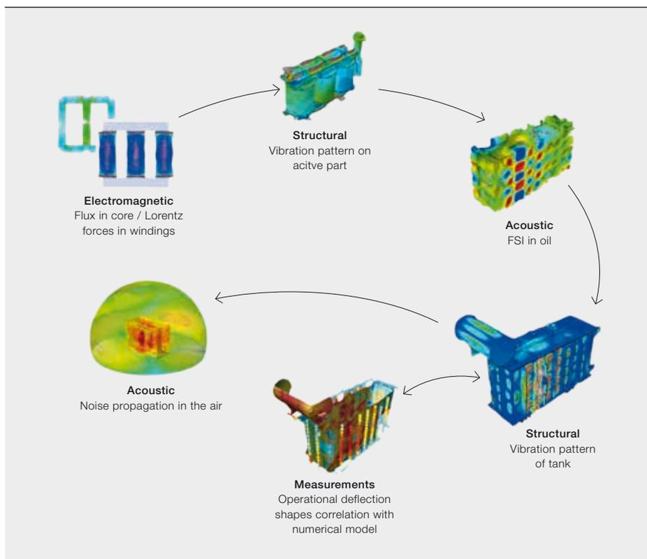
Doppler vibrometry (LDV) can be helpful in this procedure. The LDV technique is able to provide the 3-D vibration patterns of the transformer during load or no-load conditions creating so-called operational deflection shapes (ODSs) → 5 [9]. The ODS patterns can be directly compared to the numerical analysis and if necessary some improvements of the model can be introduced.
