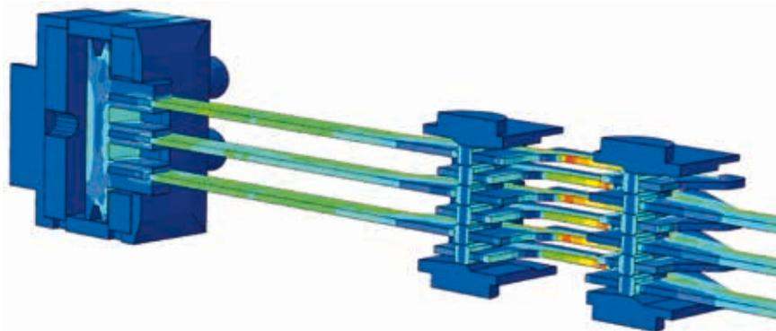
As a first step of the simulation, the pre-tensioned springs and bolts are set to an initial state. In the second step the Thomson coil load is applied as an induced force onto the area of the armature that faces the coil. On the opposite side of the armature facing the travel direction, a damping force is applied depending on the speed and position of the armature.
