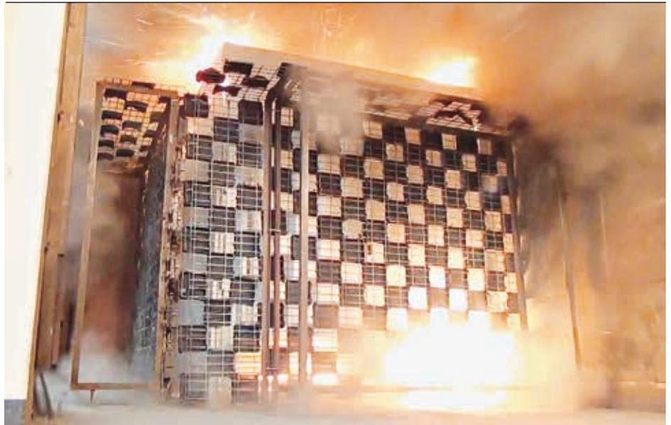
room pressure measurement. Therefore it is only possible to evaluate the pressure rise in a building by calculation. Another application for the calculation program is to simulate the pressure rise for different filling gases, ie, SF<sub>6</sub> and air. For validation, tests were conducted together with RWTH Aachen and TÜV Nord Systems GmbH.
