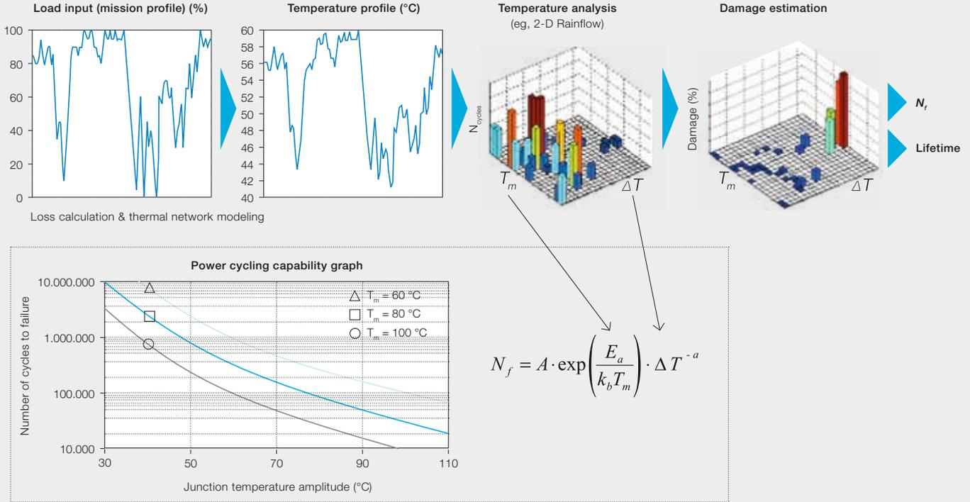
Since this failure mode is well understood, manufacturers provide cycling capability graphs for their IGBT modules. These can be used as basis-of-lifetime simulations using the following steps.
