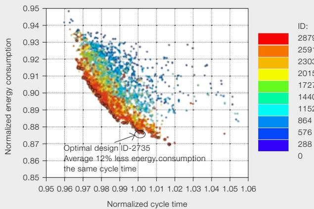
Energy-efficient design is a requirement rapidly gaining importance and one that can be evaluated using virtual prototyping. The objective is to select the drive-train control parameters, eg. allowable torques, and speed, that will minimize energy consumption at the same time that the cycle-time is minimized [3]. The problem is formulated into a multi-objective optimization problem with the drive-train control parameters as design variables and the following two conflicting objectives:
