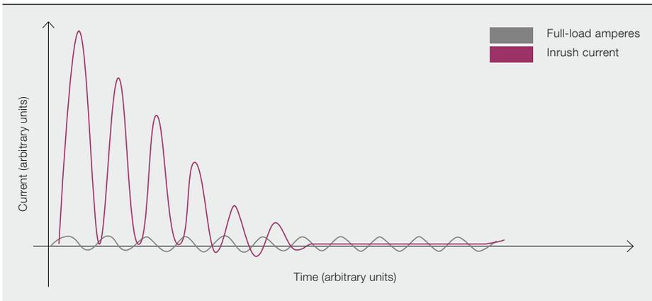
the transfer so the flux does not exceed the saturation point of the transformer's core. Energizing a transformer results in a potential peak inrush current of 5 to 12 times full-load ampacity (FLA); transferring between out-of-phase sources results in a peak inrush current of up to 20 times FLA → 7.
