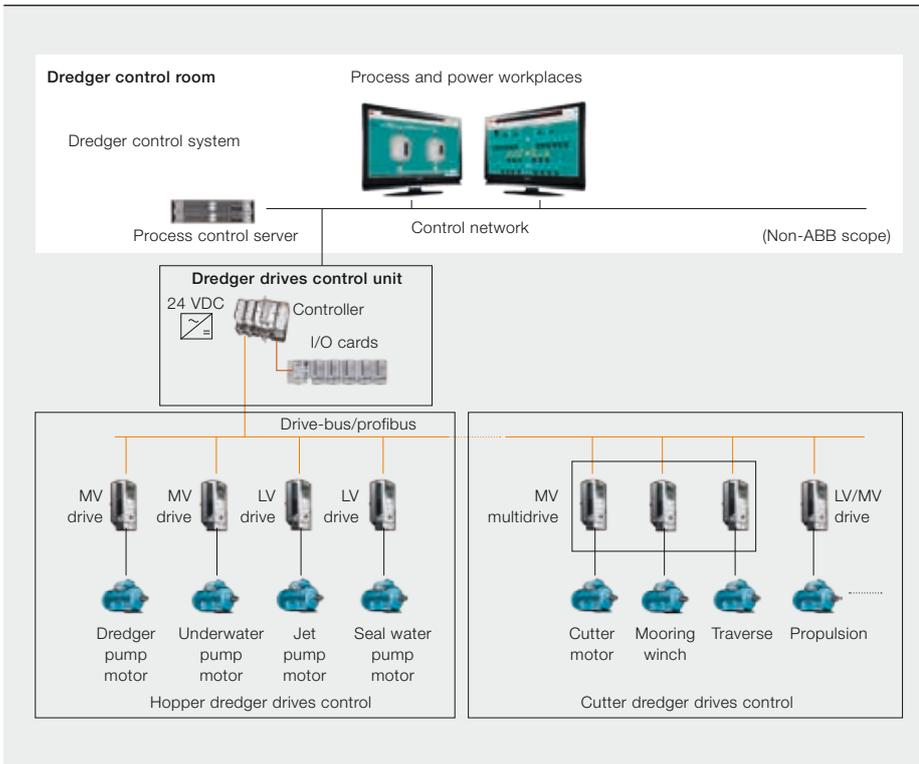
The current DreDCU application software is a standardized and scalable software package based partly on the existing software library of the AC 800M.
