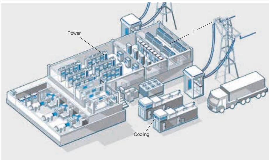
contain storage. This infrastructure is where the main functions of the data centers are implemented and the IT services are delivered. A large variety of software, virtualization, databases, web hosting, operating systems, and clouds run in data centers.
